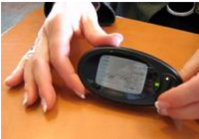
The DexCom STS continuous glucose monitor displays a chart of blood sugar readings for the previous nine hours and sounds alerts when readings go outside the
