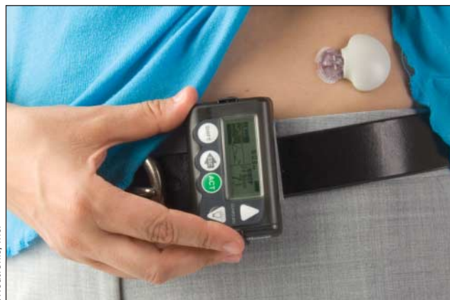
A continuous glucose monitor makes frequent measurements that provide patients an opportunity for improved glycemic control.
